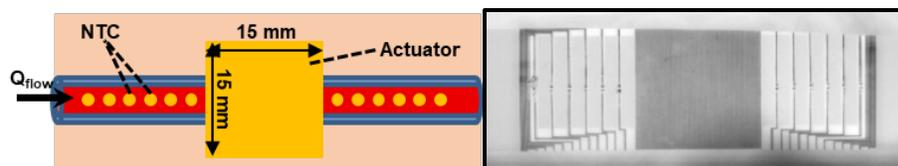
Figure 3. 15 mm by 15 mm Actuator with NTC Sensor Spacing
