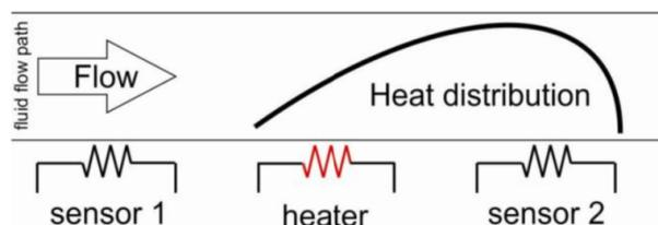
Figure 1. Depiction of Thermal Anisotropy Concept [1]
