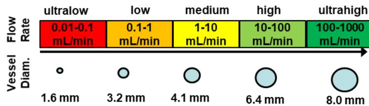
Figure 2. Variable Vessel Diameter and Flow Regimes
